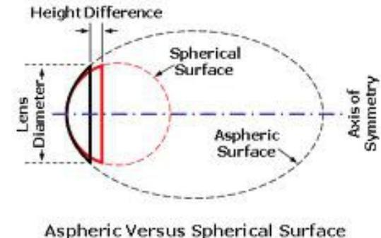
Aspheric Versus Spherical Surface
